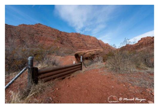
Barrier on a hiking trail, designed to keep Mojave desert tortoises out of an area, St. George, Utah. Hikers may step over this barrier to continue on the trail, while tortoises cannot gain access to the road on the other side.
