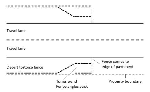
**Figure 2:** Fence-end configuration with a split fence-end. One end forms a turnaround, the other end comes close to the edge of the pavement. **While 90° angles are shown here, the fence angles for the Mojave desert tortoise should be no sharper than <b>120°** (Pers. com. Kerry Holcomb, US Fish and Wildlife Service).
