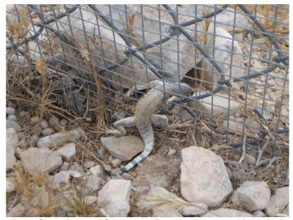
A lizard that got stuck in a fence designed for Mojave desert tortoises, and later died. The mesh size of this fence (e.g.  $1 \times 1 \text{ cm}$  (0.25  $\times 0.25 \text{ inch}$ ) is smaller than the recommended mesh size (1 inch horizontal, 2 inches vertical). Copyright Kristi Holcomb, Nevada Department of Transportation.
