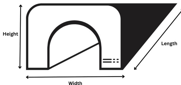
Figure 14. Crossing structure terminology illustrating structure dimensions.
