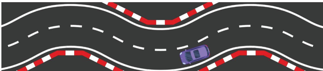
Figure 49. A chicane where curbs are placed in a straight road to make it more sinuous.
