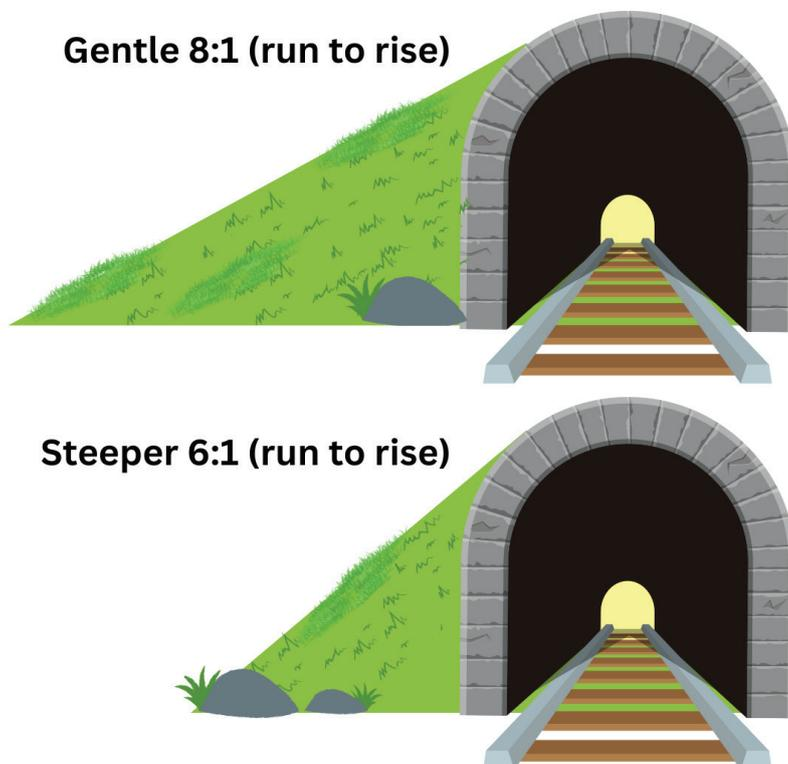
Figure 13. Approach slope visualisation of different backfill slopes approaching overpasses.
