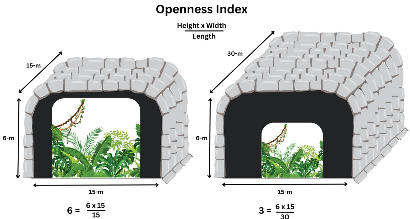
Figure 12. Openness Index visualisation illustrating the impact of length through underpasses with the similar height and width dimensions on perceived openness to elephants.
