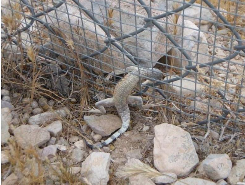
A lizard that got stuck in a fence designed for Mojave desert tortoises, and later died. The mesh size of this fence (e.g. 1 x 1 cm (0.25 x 0.25 inch) is smaller than the recommended mesh size (1 inch horizontal, 2 inches vertical). Copyright Kristi Holcomb, Nevada Department of Transportation.
