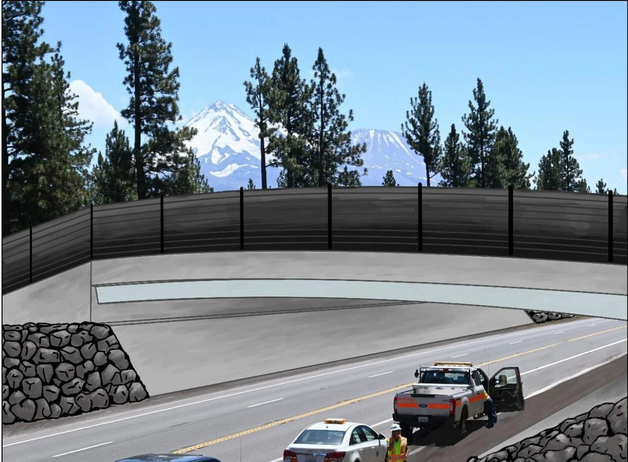
Figure 16: Rendering of US-97 FRP wildlife overpass with Mt. Shasta in the background (from Bell et al. 2022)
