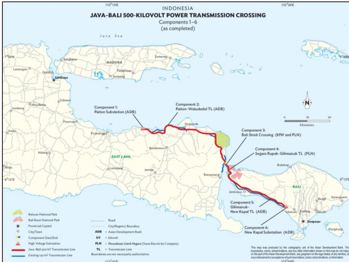
Figure 22: Location and description of the components 1 to 6 of the Java-Bali 500-kV project. Source: Asian Development Bank. Indonesia: Java-Bali 500-kV Power Transmission Crossing Project. Completion Report. February 2021.
