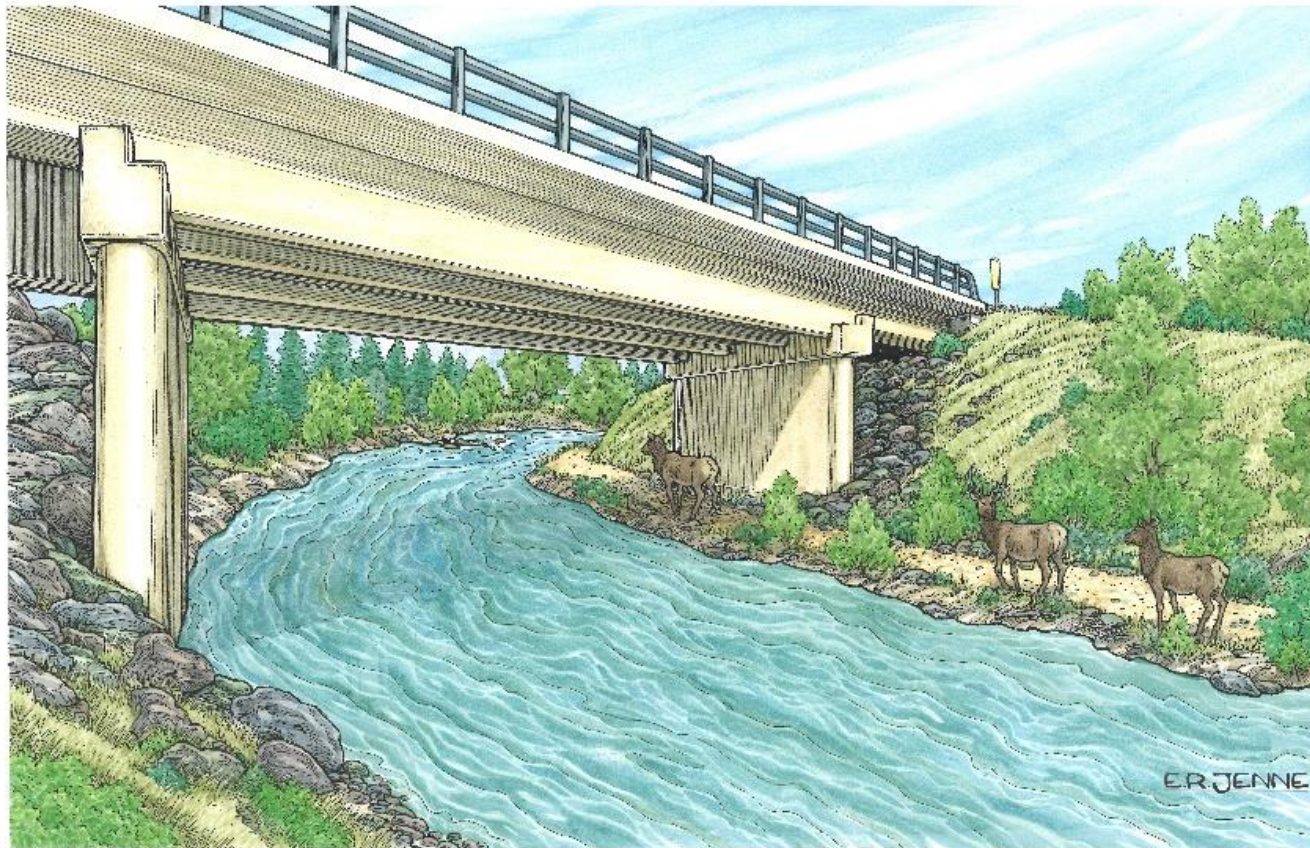
Figure 17: Rendering of a recommended bridge modification to include a walkway for safe wildlife passage. The existing bridge has no space beneath it to allow animals to walk under the bridge, which forces animals moving along the riparian corridor to cross the road at-grade. Artist rendering by Ed Jenne.
